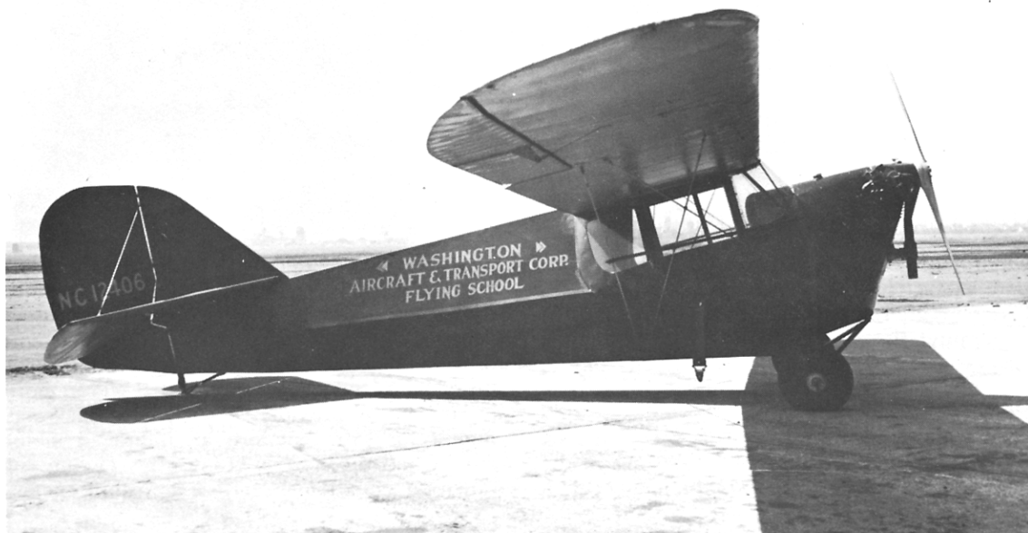
Fig. 299. Aeronca C-3 with 36 h.p. Aeronca E-113 engine.
