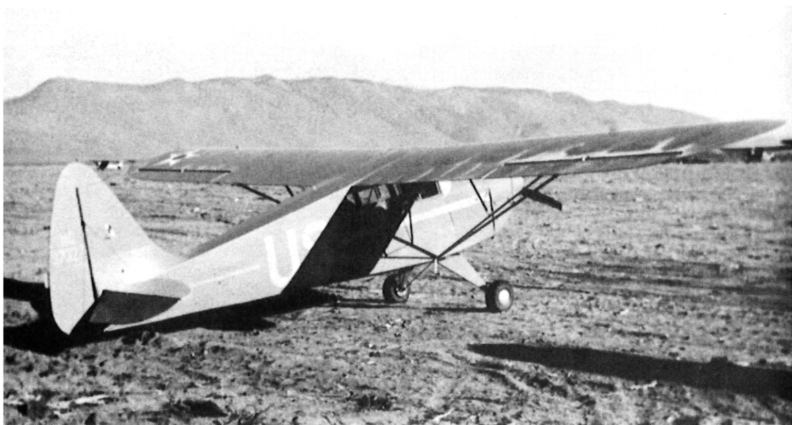
A "Cadet" on west coast at Reno Ranch; later models had balanced rudder.
