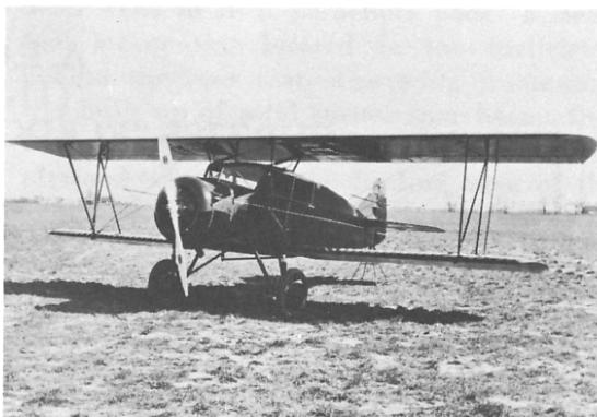
Fig. 209. Early "Cabinaire" carried four on 110 H.P.; neat installation of N.A.C.A. cowling contributed heavily to performance.
