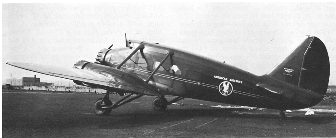
Fig. 201. The unique "Model A" was the best and the last "tri-motor" by Stinson.
